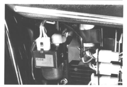
Connect an ohmmeter to the starter relay switch terminals.
