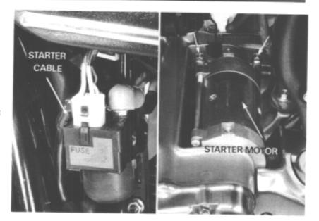
Remove the starter motor cover and starter motor.
