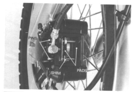
Install new brake pads with the shim on the piston side of the pad. Install the pins and clip.
