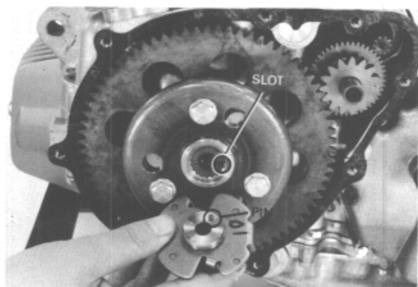
Install the spacer aligning the tangs with the holes, and tighten the advancer lock bolt to the specified torque.
