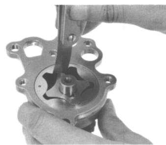
Measure the pump body clearance. SERVICE LIMIT: 0.35 mm (0.014 in)
