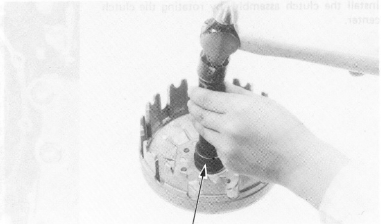
ATTACHMENT 32 x 35 mm 07746-0010100 PILOT 25 mm 07746-0030200
